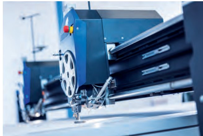
▲ Automatic thread cutter
